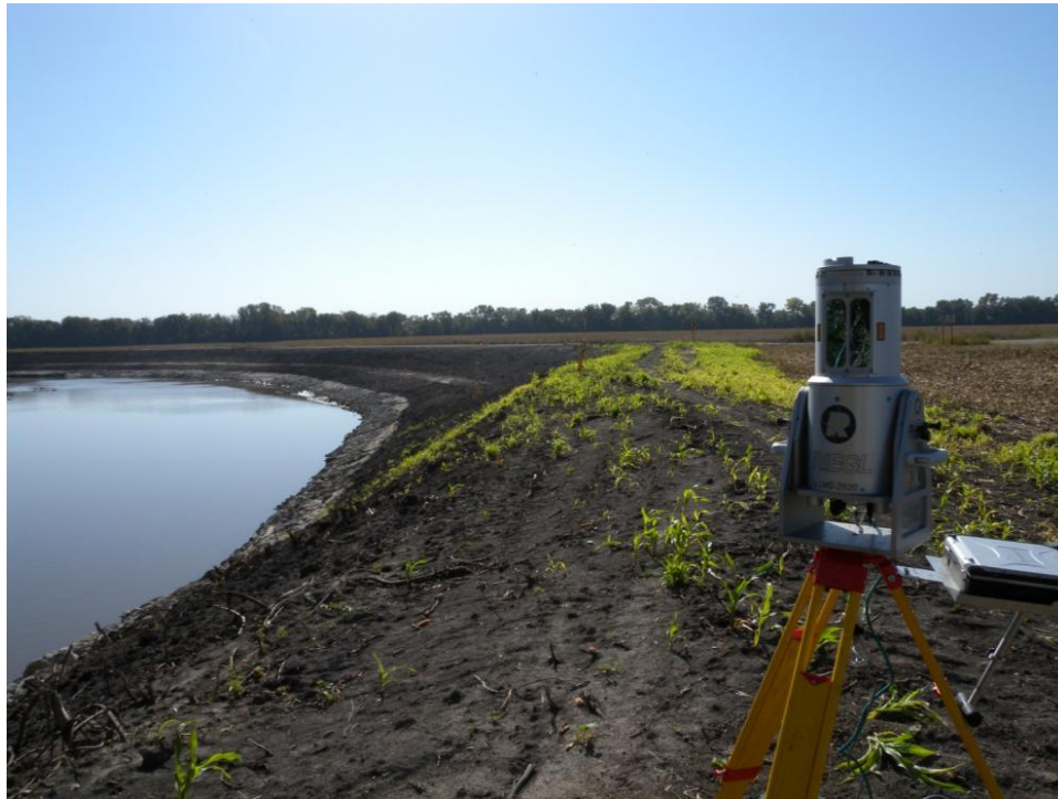
FIGURE 3.2 The Riegl LMS-Z620 Terrestrial Laser Scanner at Site 25
