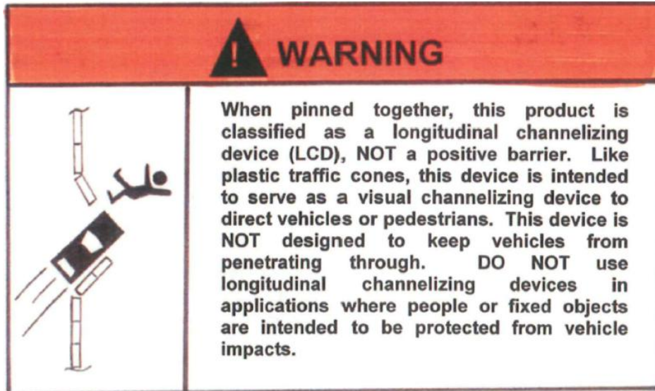
FIGURE 10 Recommended Ballast-Filled Channelizing Device Warning
