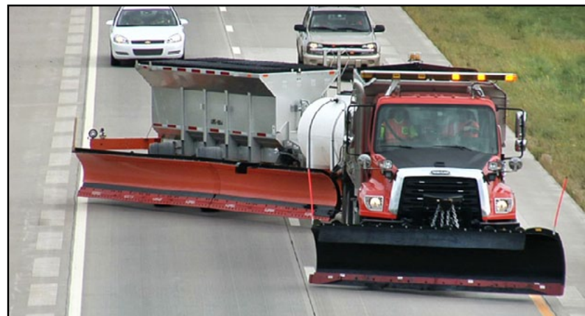
Above, the tow plow swings out to the right side, allowing it to cover a second lane of highway. At right, District Maintenance Engineer Michael Terry, is interviewed by Gardner Royce of KWCH at a tow plow demonstration in Colby on Nov. 9.
