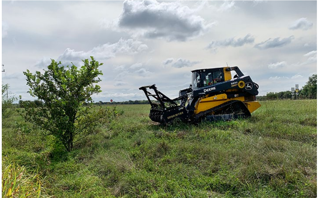
The forestry head at work on K-15, above, and on K-55, below. Photos by Greg Dixon and Scott Kent, District Five
