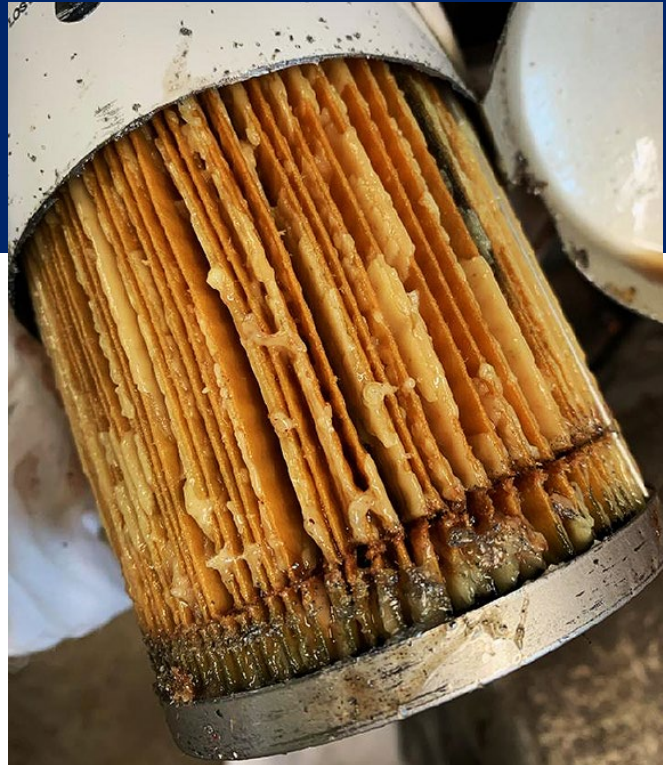
A fuel filter with diesel residue turned to gel by the frigid cold. Photo by Marty Eshelman, District Five
