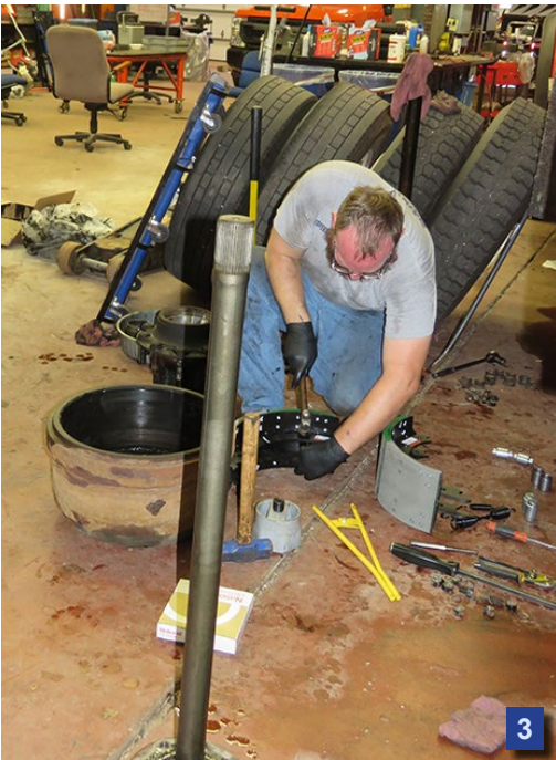
1. Equipment Mechanic Robin Walker repairs hydraulics in the District Six shop. 2. Equipment Shop Supervisor Osvaldo Erives drives in the seals on the wheels and Lorenzo Ruiz-Hernandez, Equipment Mechanic, installs the hubs as part of wheel seal job. 3. Mechanic Specialist Jeremy Neeley preps brakes for the wheel seal job. 4. Lorenzo Ruiz-Hernandez, Equipment Mechanic and Eli Ruiz-Hernandez, Equipment Mechanic square up the corner on a tailgate they are fabricating. Photos by Lisa Knoll, District Six
