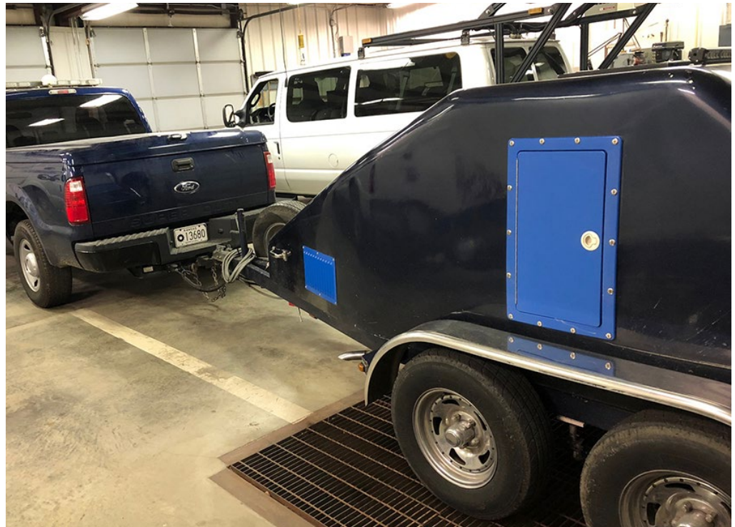
An FWD is pulled by a KDOT truck and stops and takes measurements every tenth of a mile. Photo by Rick Miller, Headquarters
