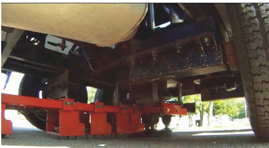
The underside of an FWD. Photo by Curtis Eichman, Headquarters
