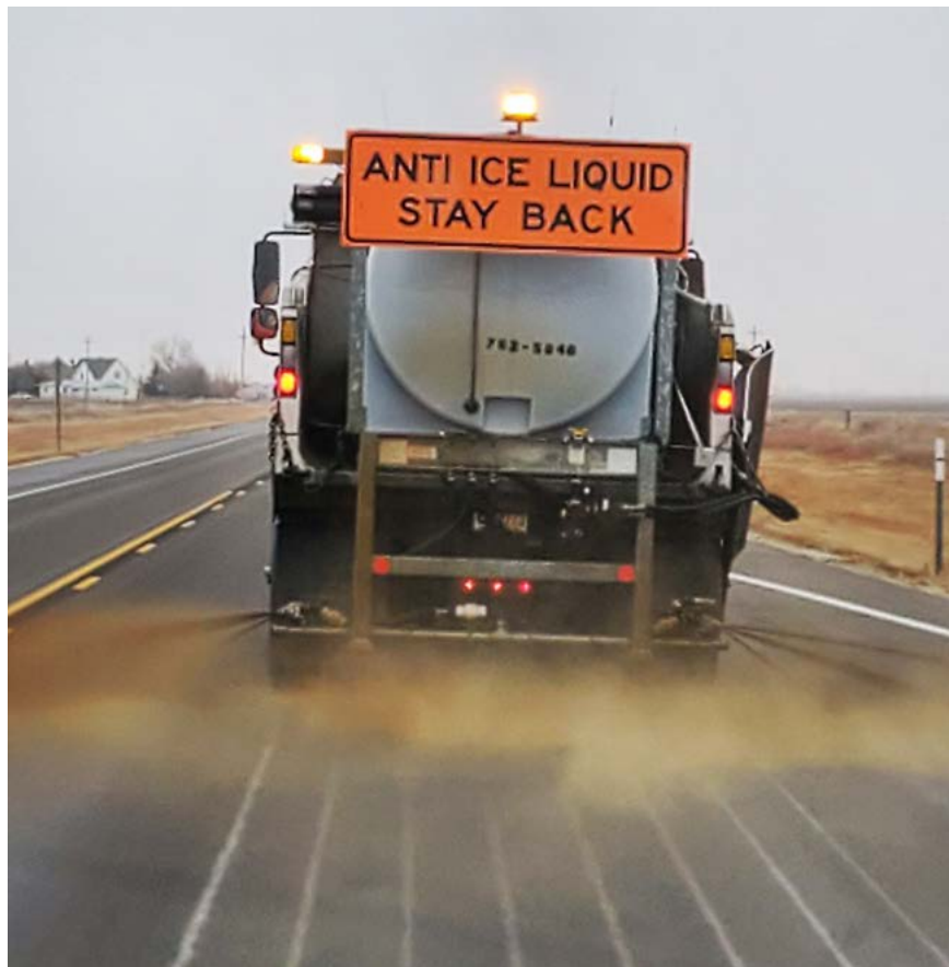
A KDOT truck sprayed a brine/beet mix on U.S. 56 between Larned and Pawnee Rock recently in anticipation of possible ice and snow. Beet juice helps brine stick to pavement. Photo by Tim Potter, District Five
