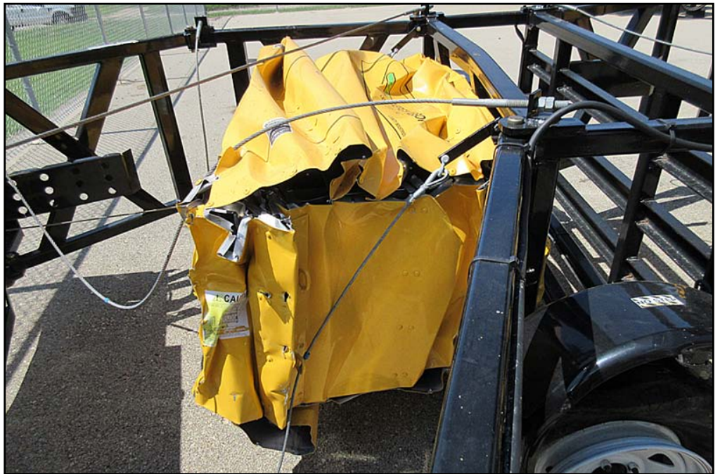
An example of an attenuator that absorbed the impact of a crash, protecting the workers, motorists and equipment. File photo
