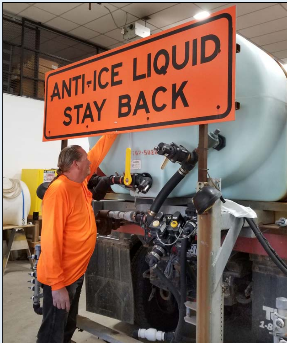
Above: David Alexander, Equipment Operator Senior with District Five, replaced a "sight tube" -- used to monitor how much brine remains in the tank. Below: Alexander stands with one of the trucks used to clear the roads. Photos by Tim Potter
