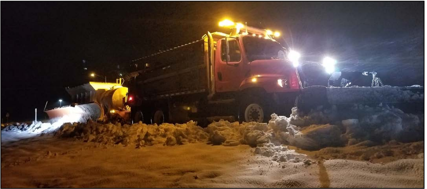
Plowing continued through the night on Jan. 11 as seen in this photo taken by Supervisor Brian Link along a northbound I-35 ramp in Johnson County. The tow plow can be seen behind but is not deployed because of the width of the ramp at this location.
