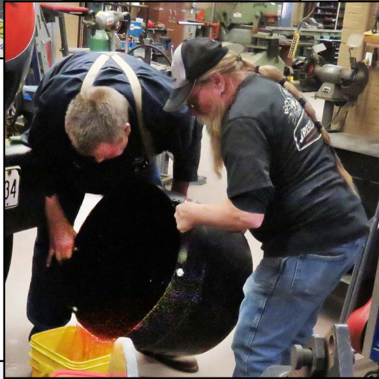
Above, Mechanic Osvaldo Erives works on a DEF system while at right, Mechanics Robin Walker and Larry Fears transfer antifreeze from a truck so they can repair the engine turbo.
