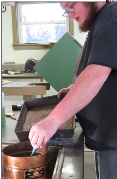
Far left, sand is delivered to the Garden City Subarea. Left, Engineering Technician Jonathon Lundin tests the sand to make sure it meets KDOT standards.
