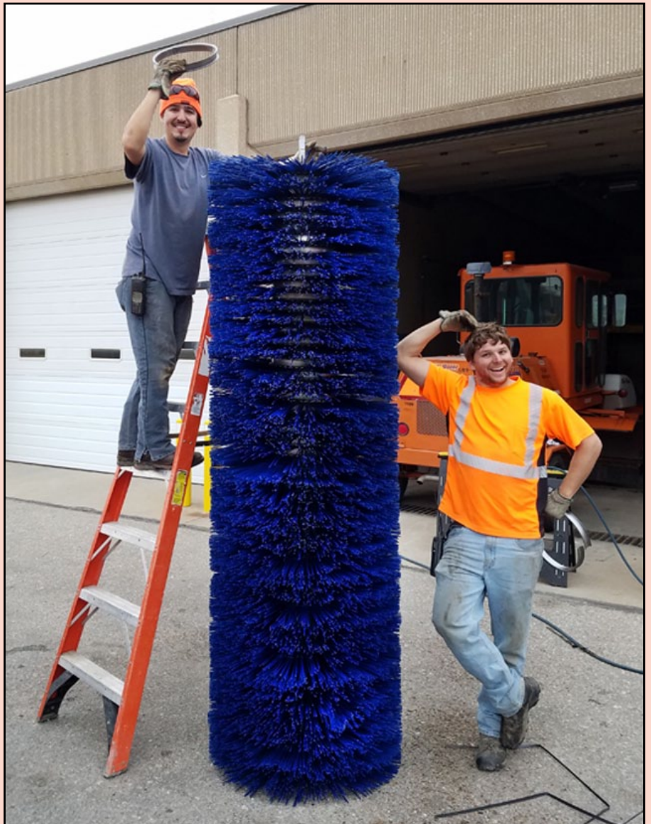
KDOT Wichita-west employees Michael Bustos and Justin Logan were in the holiday spirit while replacing the bristles on the belly broom as they thought it looked a little like a Christmas tree.
