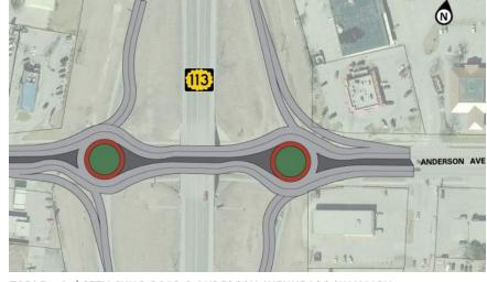
Option 2040 No Build Modified Diamond Roundabout (Elliptical)
