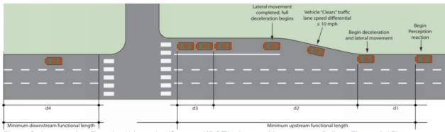
Figure 8: Intersection Functional Lengths (Source: KDOT's Access Management Policy, Figure 4-17)
