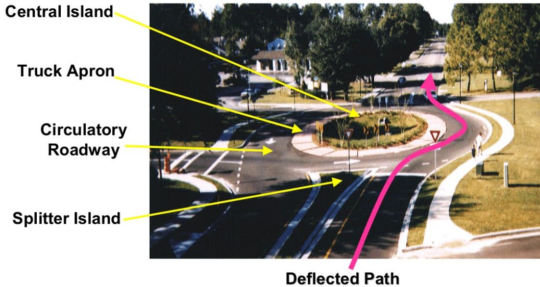
Exhibit 1-9 Elements of a Roundabout
