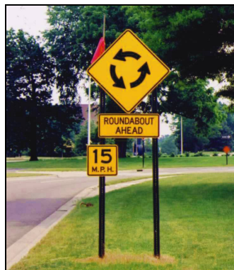
Exhibit 2-3 Roundabout Ahead Warning Signs.
