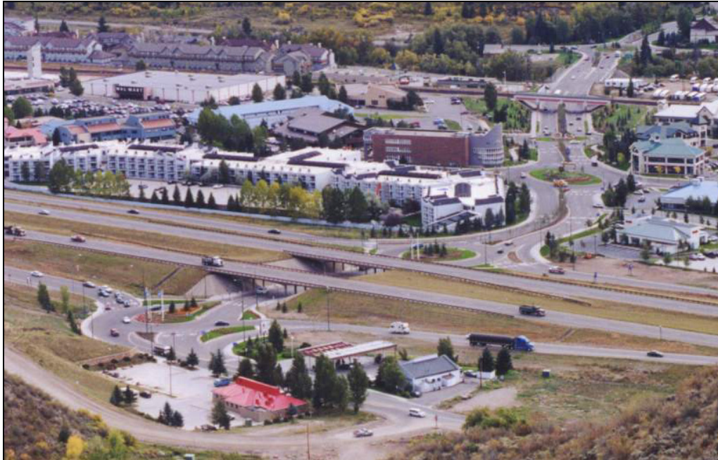
Exhibit 8-4 Roundabouts in Series (Avon, Colorado)
