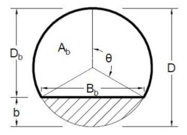
The values of  $D_b$ ,  $B_b$ ,  $P_c$ ,  $P_b$ , and  $A_b$  all depend only on the pipe diameter, D, and the embedment depth, b. However, the relations for  $B_b$ ,  $P_b$ , and  $A_b$  can be expressed most compactly in terms of the angle  $\Theta$  defined in Figure 6.2.4-1. The angle  $\Theta$  depends only on the ratio b/D. Its value in radians is computed with the equation below.
