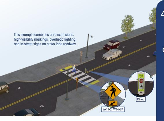
This group of countermeasures includes improved lighting, advance or in-street warning signage, pavement markings, and geometric design elements. Such features may be used in combination to indicate optimal or preferred locations for people to cross and to help reinforce the driver requirement to yield the right-of-way to pedestrians at crossing locations.
