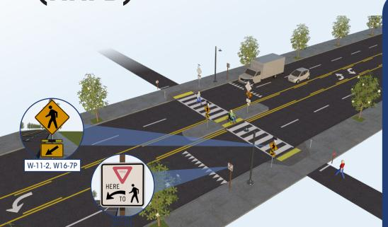
RRFBs are pedestrian-actuated conspicuity enhancements used in combination with a pedestrian, school, or trail crossing warning sign to improve safety at uncontrolled, marked crosswalks. The device includes two rectangular-shaped yellow indications, each with an LED-array-based light source, that flash with high frequency when activated.
