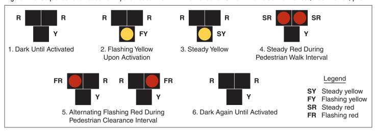
When a pedestrian activates a PHB, a flashing yellow light is followed by a solid yellow light, alerting drivers to slow. A solid red light requires drivers to stop while pedestrians have the right-of-way to cross the street. When the pedestrian signals display a flashing DON'T WALK indication, the overhead beacon flashes red, and drivers may proceed if the crosswalk is clear.
