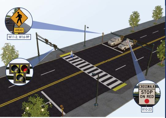
A Pedestrian Hybrid Beacon head consists of two red lenses above a single yellow lens. Unlike a traffic signal, the PHB rests in dark until a pedestrian activates it via pushbutton or other form of detection. When activated, the beacon displays a sequence of flashing and solid lights that indicate the pedestrian walk interval and when it
