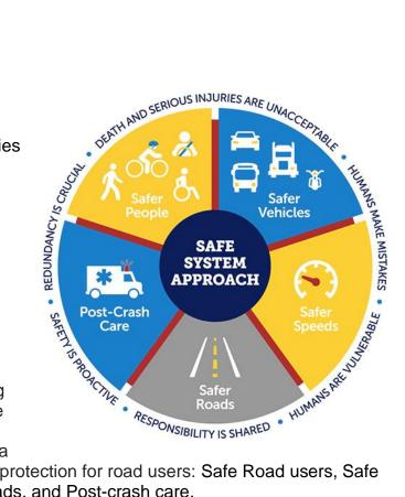
holistic approach with layers of protection for road users: Safe Road users, Safe vehicles, Safe speeds, Safe roads, and Post-crash care.
