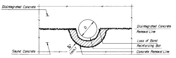
(b) All Reinforcing Bars Other Than the Top Layer of Transverse Bars. Where more than  $\frac{1}{2}$  the diameter of the steel is exposed (FIGURE 731-3), or where the bond between existing concrete and reinforcing steel has been destroyed (FIGURE 731-2), remove the concrete adjacent to the bars to a depth that shall permit concrete to bond to the entire periphery of the bar with a minimum clearance of  $\frac{3}{4}$  inch.
