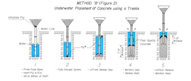
Method B (Figure 2): Use a tremie tube, with a pig separating the ground water and concrete, to place concrete into the shaft. Once the tremie tube is resting on the bottom of the shaft, install the pig just below
