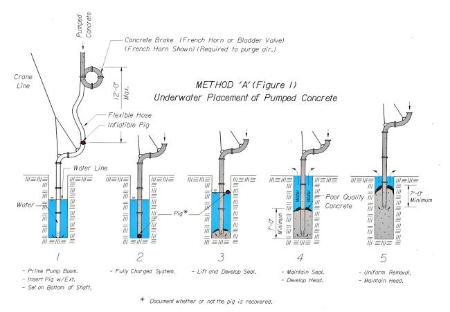
**Method A (Figure 1):** Use a pump and extension tube, with a pig separating the ground water and concrete, to place concrete into the shaft. Install a concrete brake (e.g. bladder valve or French horn) at the end of the pump boom to purge the air from the pump line. Fully charge the boom with concrete (no air gaps) then install the pig in the top of the extension tube.
