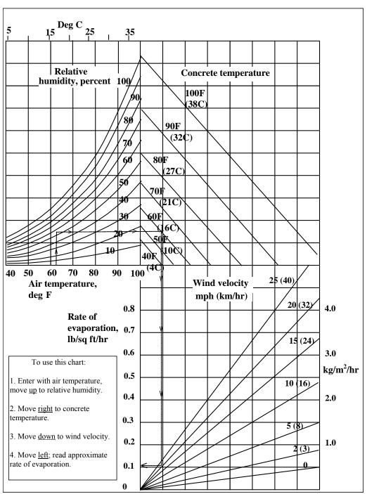
FIGURE 710-1: STANDARD PRACTICE FOR CURING CONCRETE
