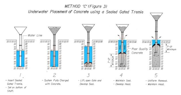
**Method C** (**Figure 3**): Use a tremie tube, with a sealed gate separating ground water and concrete, to place concrete in the shaft. Fully charge the tremie tube and hopper, then raise the tremie tube by 1 tremie diameter and seal the discharge end of the tremie tube with the fresh concrete.
