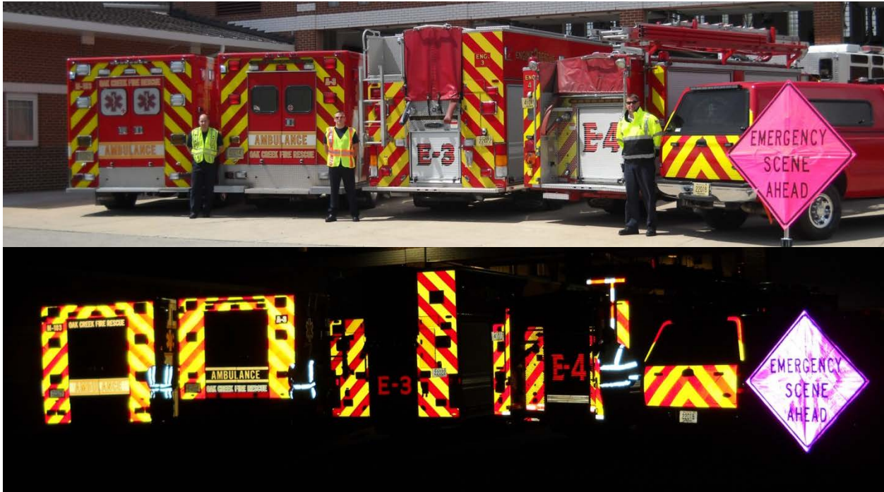
Figure 3: Emergency Vehicles with Retroreflective Chevron Striping (Photo Courtesy of the City of Oak Creek Fire Department, WI)
