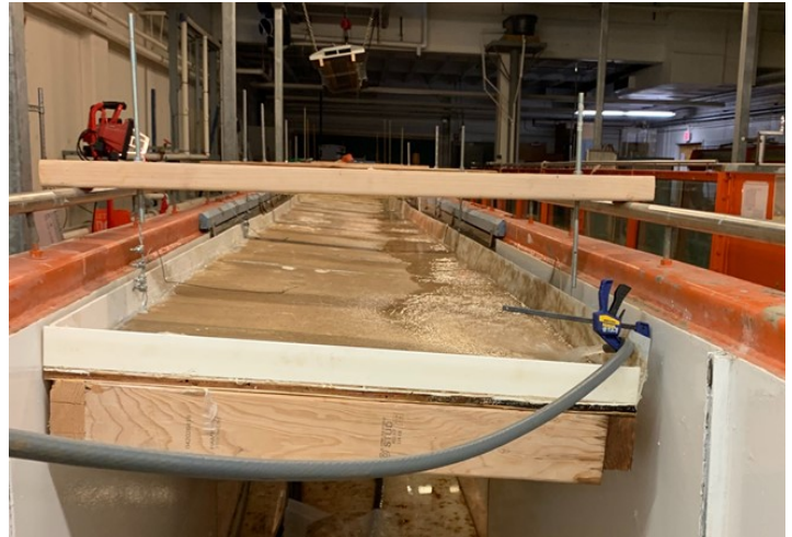
Single Inflow from the High Side of a Scale Bridge Deck Model
